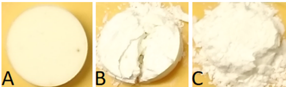
Figure 6 - Photographs of sintered ceramic specimens based on their integrity levels (examples from the sintered samples). (A) Intact (TZ-3YSB-E_1M). (B) Partial fracture (3-97 [%wt] with monoclinic Nb 2 O 5 ). (C) Total fracture (10-90 [%wt] with monoclinic Nb 2 O 5 ). Sintered from green specimens diameter: 11 mm.
